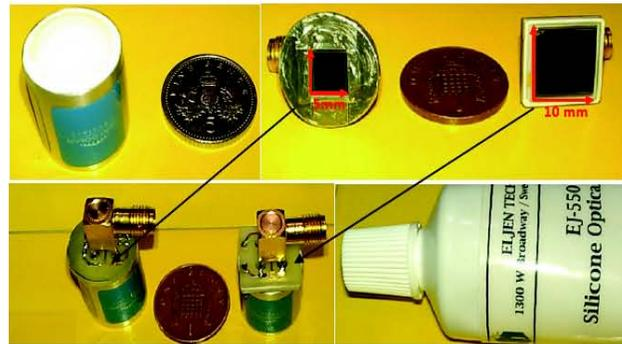
**Figure 6. LaBr<sub>3</sub> detector and the 5x5 mm and the 10x10 mm APD sensors used for measurements**
