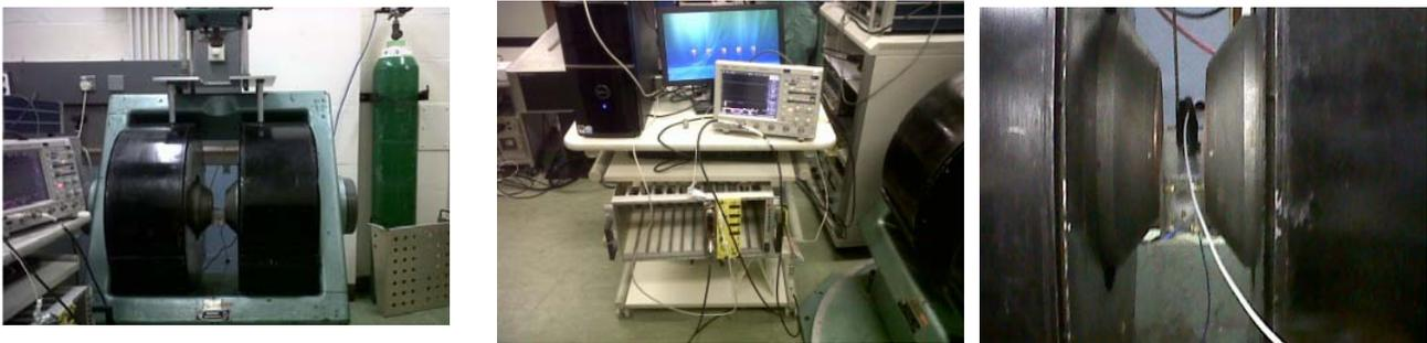
**Figure 9.** The 1T Magnet, used for the study. The detector set-up can be seen in between the pole pieces in the bottom right figure.
