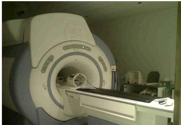
**Figure 11. The 3T MRI magnet at the York Neuroimaging Centre. The detectors are placed on the side of circular cage shown in the centre of the magnet. The cables from the detectors can be seen stretching along the bed**
