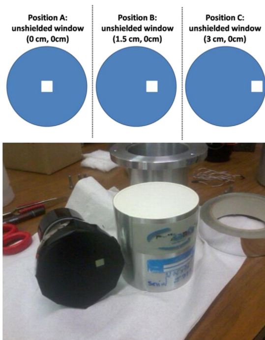
Fig. 8. In the top panel the positions (labeled A, B and C) of the three windows on the photocathode entrance window are represented. The photo shows the \text{LaBr}_3:\text{Ce} crystal and the shielded PMT. The window is at 1.5 cm from the center along the x-axis (position B).
